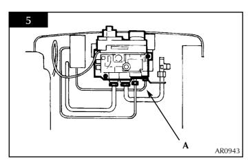
2.3 Loosen main injector nut on airbox and disconnect from injector, see diagram 6, A.
